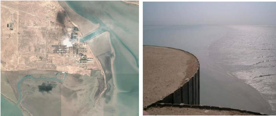
Figure 9-4 Left: Subiyah power plant with intake structure projecting into the Khor Al-Subiya and resulting coastal morphological change on the lee of intake walls, and outfall discharge to Kuwait Bay (From Google maps, November 2016). Right: view of the sediment deposits downdrift.
